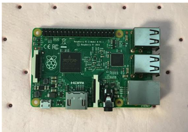
Figure 1. New developments in small, low-cost computing devices such as the Raspberry Pi (pictured) are driving advances in reaction control strategies.
